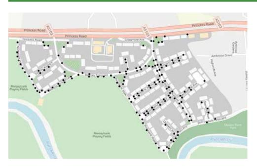
In August we carried out a survey of the grids on the estate and found most of them to be blocked and full of leaves. The diagram shows all the drains we were able to survey. Unfortunately there were a few grids we couldn't check because of parked cars. All blocked grids have now been reported to the council.
